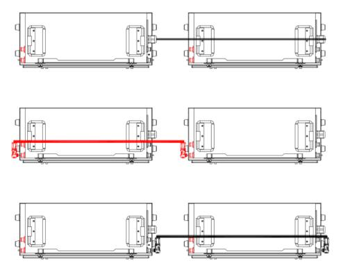
Step 9: Please connect the positive pole of one battery to another with red power cables, connect the negative pole of one battery to another with black power cables and connect one battery com port to another battery com port as the above figure shows.
