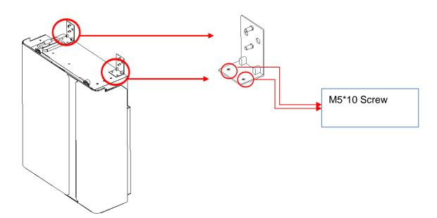
Step 2: Install the battery brackets on the battery with M5 screws.
