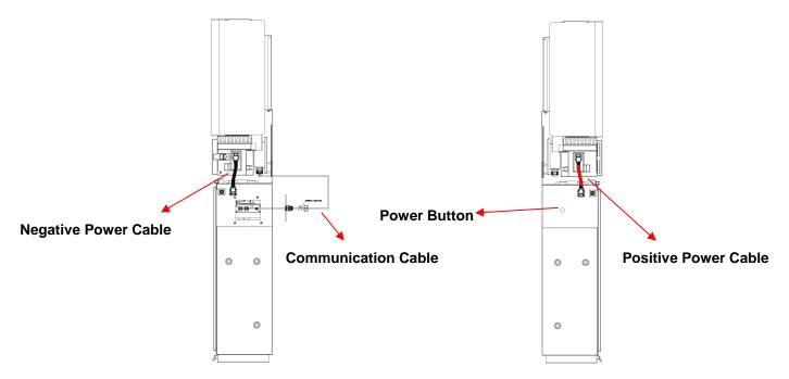
Step 6: Install the inverter above the battery, please refer to the SMILE5 Installation Manual.
