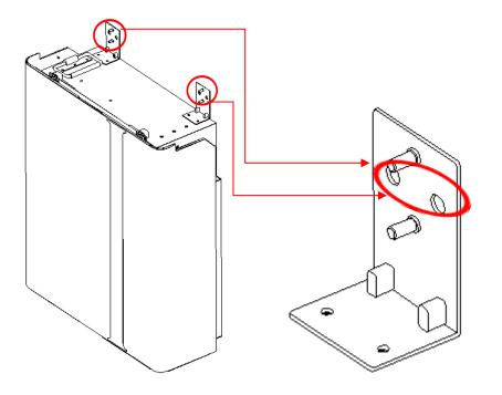
Step 3: Please drill four holes (two on each side) directly on the wall at the marking positions of the brackets with an impact drill (bit  $\phi$  8.0mm, length 20cm) and the depth of each hole should be about 7 cm.
